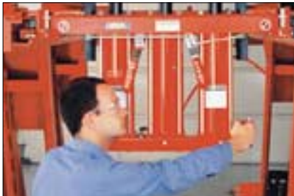
Swing Air-Jack 133-62-1 8,000-lb. (3600-kg) Capacity
